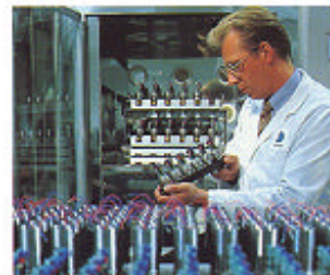
Computerized testing and calibration of pressure transducers.
