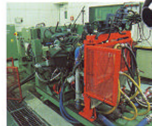
Automotive engine shown on a research and development test bed.
